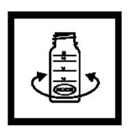
**6.** Swirl to mix. Wait eight minutes for full color development. If phosphate is present, a blue-violet color develops. Complete the test and read the result within 10 minutes of the addition of the powder.
